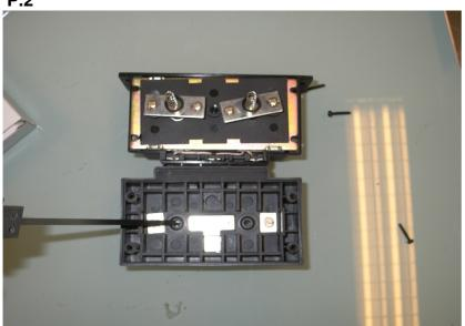
Use a phillips screw driver and cone hole just a little to make shore there are no plastic that prevent the shaft on the contactor plate to go into this hole.
